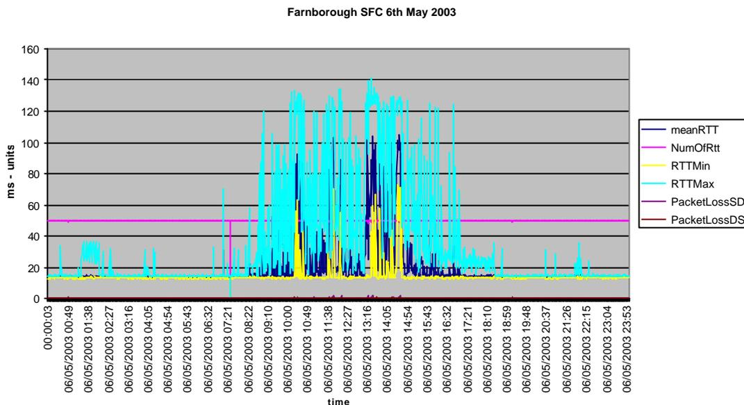
The graph shows that, while the network is fairly reliable at packet delivery (in pink), the maximum delivery time (in light blue) for those packets varies substantially during the day. Significantly it follows the working day very closely, with an increase in delay after 08:30 but dropping again after 17:00.
